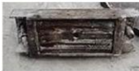
Shuttering magnet bottom debris is not cleaned
