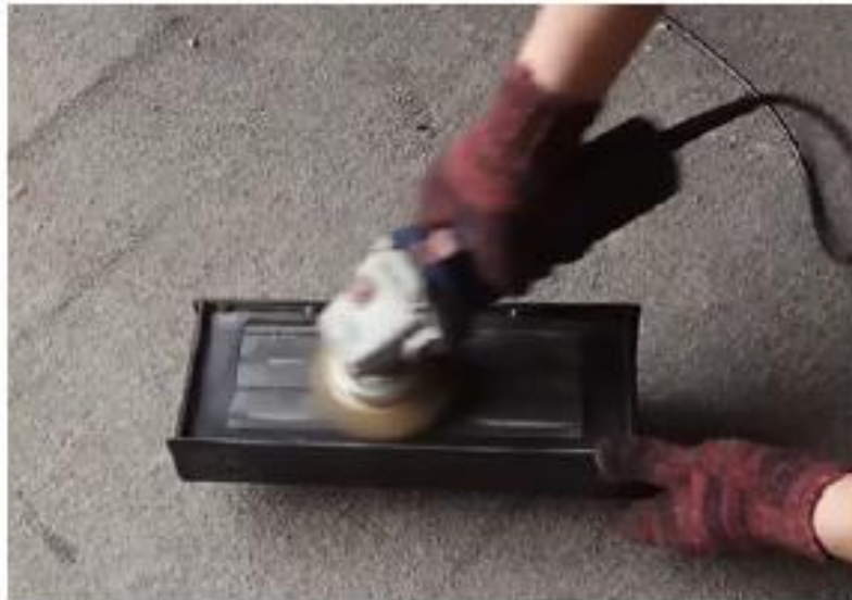
Shuttering magnet bottom debris is not cleaned
